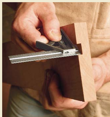
Checking the depth of a groove
