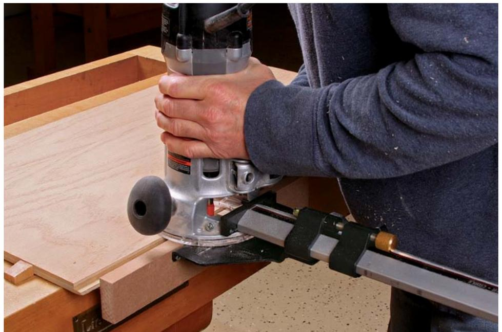
**Quick rabbets.** Teamed up with a straight bit, an edge guide makes accurate rabbets in the sides of a cabinet, to hold the back. Again, make multiple passes for best results. Note that Adams is holding the workpiece with benchdogs, which grip solidly without getting in the way.
