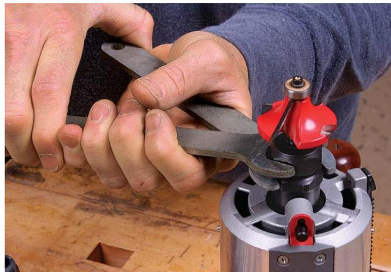
**Tighten it firmly.** Look for a router with two nuts and two wrenches for tightening the collet as shown. Routers with a spindle-lock button and one wrench are harder to hold onto as you tighten the bit.
