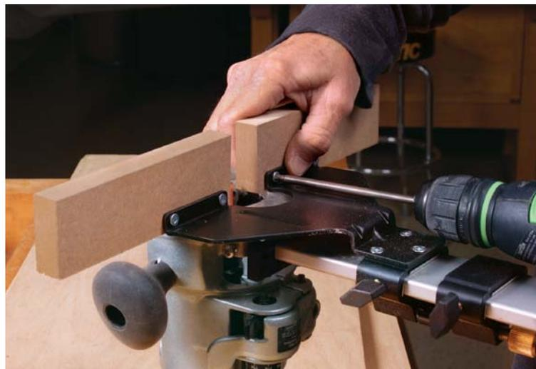
**Improve the fence.** An edge guide's short fence halves have holes for screwing on extralong pieces. This auxiliary fence adds control, helping you keep the edge guide in good contact with the work. Flat, stable MDF is great for fences.
