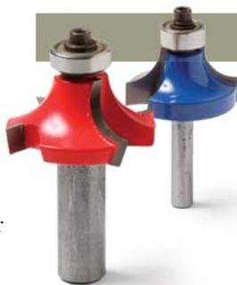
Choose a bit with the thicker shank when possible. The router will hold these more firmly. The bigger shanks also flex less, which means less vibration.
