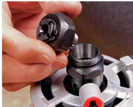
The collet grabs the bit. Not every bit has a ½-in. shank, so be sure your router comes with both ½-in. and ¼-in. collet sizes. When installing a collet, make sure its mating surfaces are clean.
