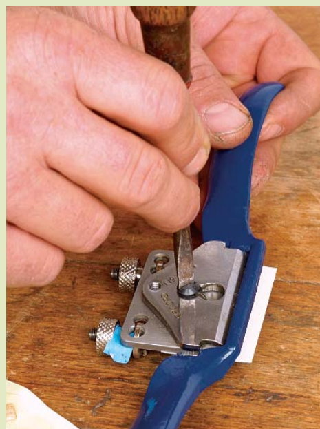
Use the stock cap iron to clamp the blade in place. The blade will create a flat bed to support it completely. Use the center screw to apply even pressure.
