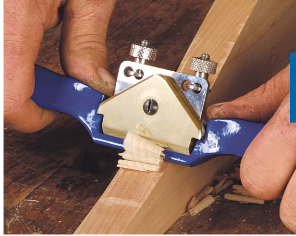
The well-tuned spokeshave. Outfitted with an after-market blade, a flat bed and a shopmade cap iron, a spokeshave—either pushed or pulled—will plane curved surfaces glassy smooth.
