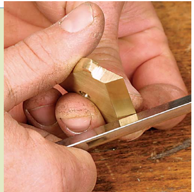
Last, burnish a very fine burr on the front edge. This will create a tight seal against the blade, preventing chips from slipping underneath. Flatten the hook slightly on a bench stone.
