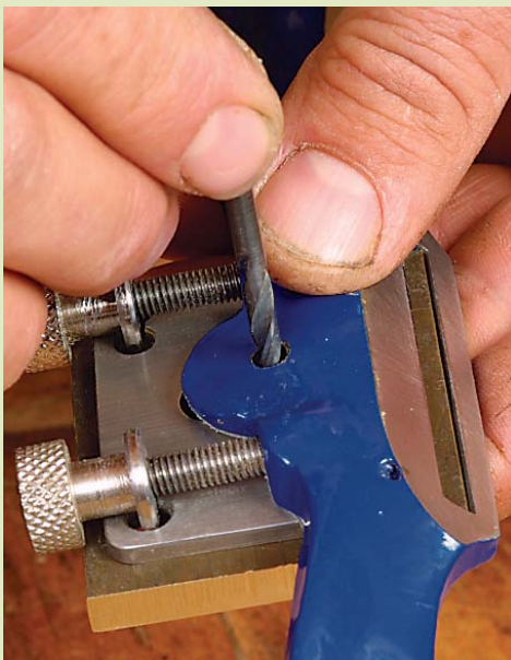
Next, mark for the center hole. This simply is a clearance hole for the center screw, which threads into the body of the tool.
