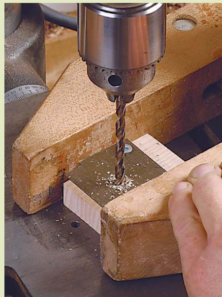
Mount the cap back onto the wood block for drilling. A screw clamp makes a good vise. Next, use the bandsaw to cut the corners off the back edge.
