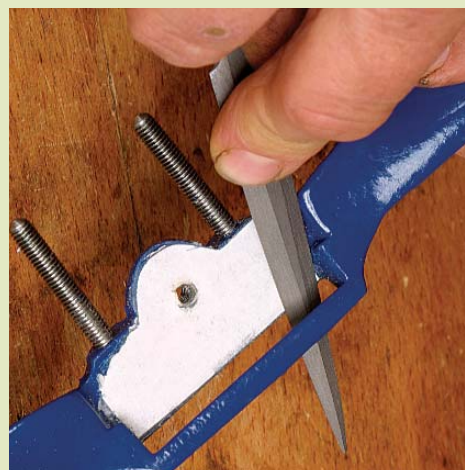
Remove excess epoxy. Some epoxy will squeeze out around the paper, but it's easy to trim and pare cleanly.
