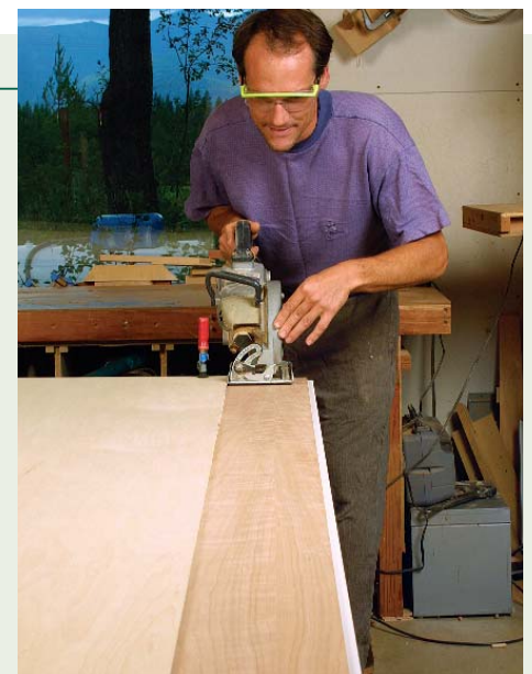
Cutting a plywood sheet. A second sheet of plywood (top) makes a serviceable edge guide for rough-cutting large sheets.
