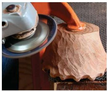
**The block becomes a bowl.** An angle grinder fitted with an aggressive Holey Galahad carbide sanding disk shapes the outside. A scrap block inside the bowl keeps the droplets above the workbench.
