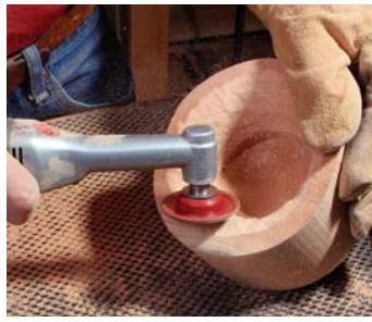
**Quick cavity.** Kamerath drills out the block with a large Forstner bit. After bandsawing it to an oval, he shapes the interior with a Proxxon mini grinder fitted with a needle-toothed carbide carving wheel.
