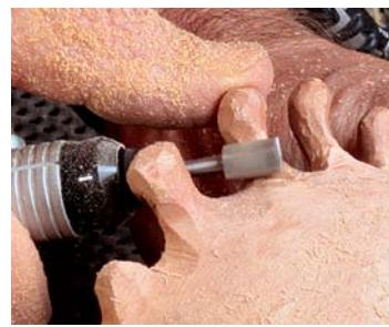
**Carving water from wood.** He refines the droplets using a Wecheer rotary tool and various bits, then finishes them with round files and sandpaper. All other surfaces are hand-sanded as well.
