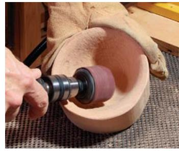
**Speedy sanding.** Using a Guinevere flex-shaft sanding system with inflatable attachments that conform to the workpiece, Kamerath can smooth any surface quickly.
