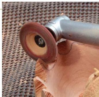
**Slots between the drops.** Following pencil lines, Kamerath uses the Proxxon grinder to cut notches between the droplets.
