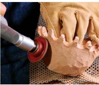
**Smoothing time.** Using the mini grinder, Kamerath fairs the roughly rounded exterior left by the angle grinder. He follows this step by smoothing the surfaces with the Guinevere sander.
