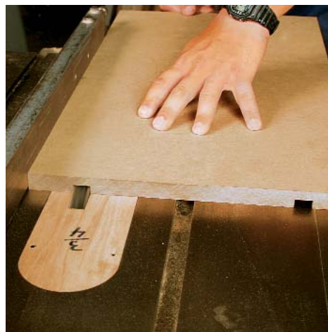
Cut some grooves. A dado head plows a pair of parallel grooves in an oversized blank.
