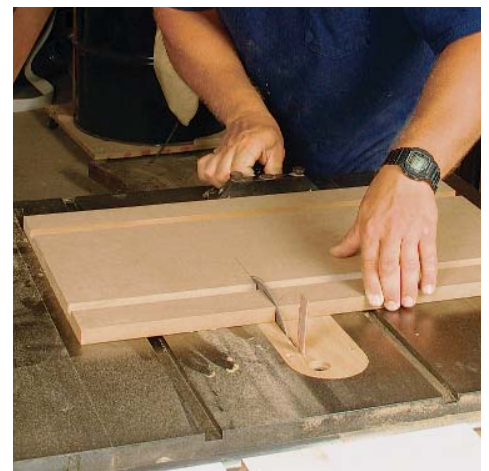
Cut the blank in two. Crosscutting the blank provides stock for the base and platform.
