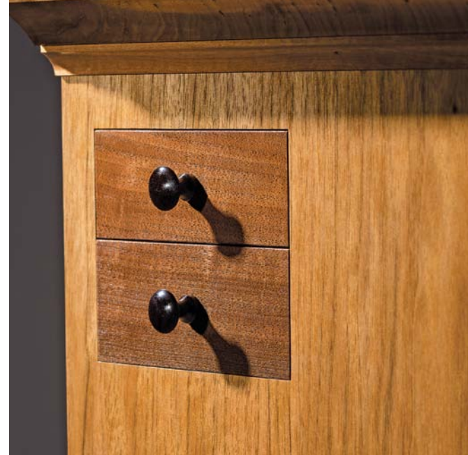
I'll have two drawers on the side. The diminutive drawers travel through a hole in the solid butternut case side and rest in their own drawer box.
