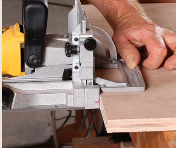
Dial in the height. The DeWalt fence is easy to adjust with a thumbscrew (left), with scales that are easy to read.
