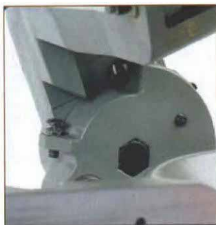
Vertical adjustments are easy. Two bolts with locknuts act as 45° and 90° stops.
