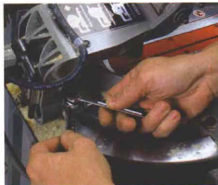
Two wrenches required. To adjust the 45° and 90° stops, you may have to tilt the saw head to access the bolts and locknuts.
