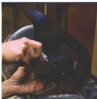
This brush is still in good shape. Worn-out brushes can lead to sparks coming from the motor, and they can indicate a loss of power. Replace brushes when they get too worn, which would be about half the size of the one shown here.
