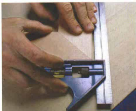
You need two pieces to test miters. Scraps at least 3 in. wide are better than narrow pieces to get a good reading on a miter.
