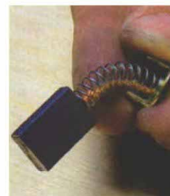
This brush is still in good shape. Worn-out brushes can lead to sparks coming from the motor, and they can indicate a loss of power. Replace brushes when they get too worn, which would be about half the size of the one shown here.
