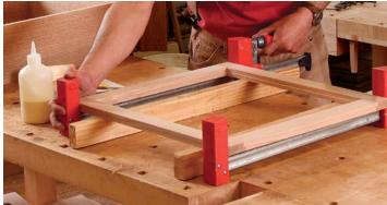
corners with chisels afterward. Instead, I cut the rabbets for the mirror in the rails and stiles first, and I joined the parts using slip tenons. This gives me a strong door with a perfectly square rabbet for the mirror.
