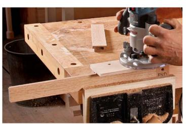
Stiles next. Butt the end of the stile tightly against the stop and tight to the top.
