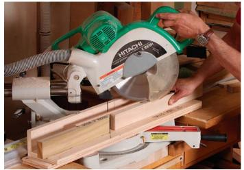
No rocking in this cradle. To turn the compound-angle miters into simple 45° cuts, Rodriguez supports the work in a cradle. He makes both left and right cuts in the front fence first, and then uses those kerfs to line up the molding cuts.
