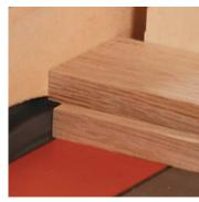
Make way for the mirror. Use the same dado set to rabbet the stiles and rails (left) and to cut half-laps in the rails (right).
