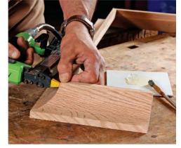
From cradle to case. After carefully cutting the miters, using the case as a guide for the length of the front piece, cut the side moldings to final length. Assemble the sections on the bench using glue and a pin nailer (above). Let the assembly dry, slide it onto the top of the case (right), and
