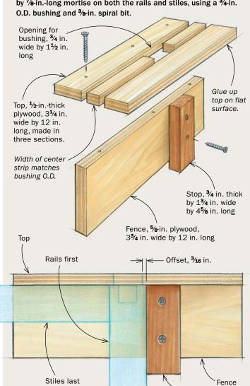
Stop locates mortises in both rails and stiles.
