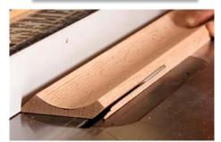
**Trim the molding.** Now make the 45° trim cuts on both edges to finish off the molding.
