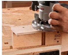
Rout the rail first. Clamp the jig in a vise, with the bottom of the rail tight against the stop and with the end tight to the top, then rout using a 3/8-in. spiral bit and guide bushing.
