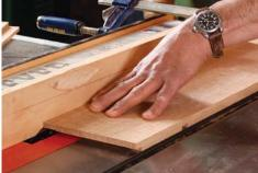
**Dadoes and bottom rabbet.** After cutting the rabbet for the bottom, cut the dadoes for the top and fixed middle shelf (left). Any tearout on the back will be removed when you cut the rabbets for the back panel and French cleat (right). Bury the blade in a sacrificial fence when rabbeting.
