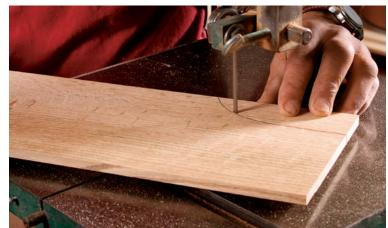
Bandsaw the bottom curve. The cutout at the bottom of the cabinet gives the case a slimmer look. Smooth the bandsaw marks with a spindle sander, a spokeshave, or curved sanding blocks.
