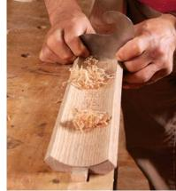
Clean up before mitering. Use a gooseneck scraper and a curved sanding block to remove the tablesaw marks.
