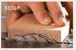
Height, then angle. Raise the blade to meet the apex, or high point, of the arc (above). Now angle the fences so that the ends of the arc align with the leading and trailing teeth of the blade. Mark that angle on the tablesaw top and then clamp the fences in place (right).
