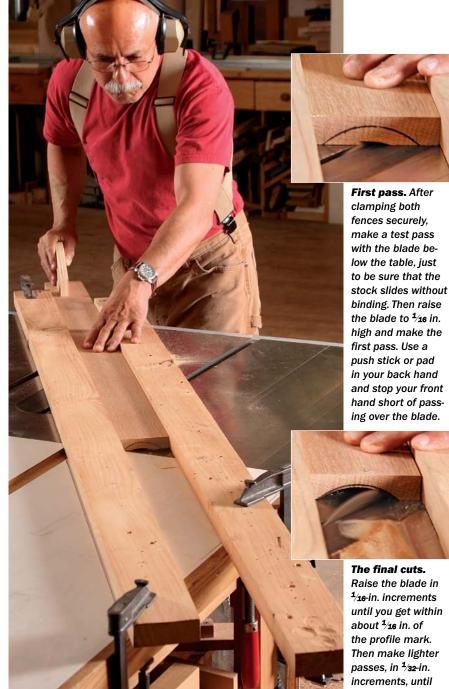
The final cuts. Raise the blade in <sup>1</sup>/<sub>16</sub>-in. increments until you get within about 1/16 in. of the profile mark. Then make lighter passes, in <sup>1</sup>/<sub>32</sub>-in. increments, until you hit the mark.
