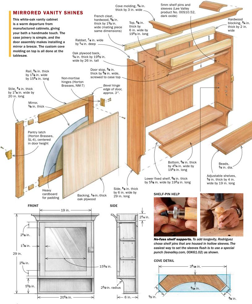
the arc on the bottom of each side. This arc gives the cabinet a slimmer look and provides more clearance to reach items stored on the bottom shelf.
