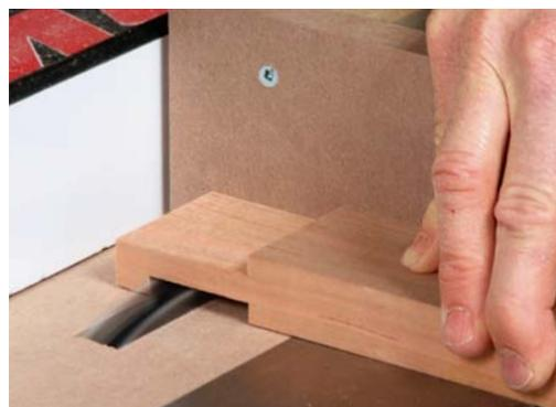
**Tenons in minutes.** Set the rip fence to position the first cut at the shoulder (above), and make a series of nibbling cuts (center left) to finish the job. To cut the top and bottom of the tenon, change the height of the blades if necessary and just flip the workpiece on edge (bottom left).
