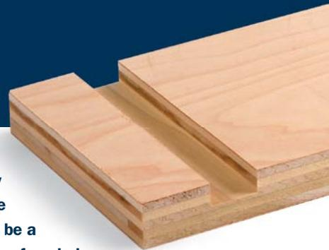
A dado is a groove cut across the grain and is usually sized precisely for a second piece to fit into. Since dados are crosscuts, tearout can be a problem without a zero-clearance surface below the cut. If the back edge will show, you'll need zero clearance there, too. You can use a variety of fences to make a dado cut safely, but it depends on the size of the workpiece and location of
