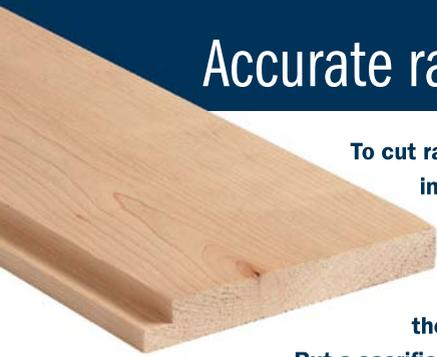
To cut rabbets, you should bury the dado set in a sacrificial rip fence. This makes it easy to adjust the width of the rabbet: You simply nudge the fence a bit instead of fine-tuning the width of the dado stack.
