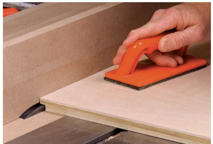
**Fast, accurate rabbets.** Whether the rabbets are along the edge (left) or end of a workpiece (above), you can run the workpiece against the fence. But you'll need a zero-clearance throat plate to prevent tearout when working across the grain. Push pads do a good job controlling the workpiece, but you'll need to support narrow workpieces with the miter gauge.
