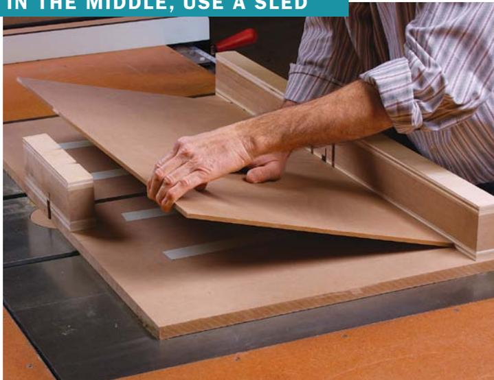
**Refresh your crosscut sled.** To prevent tearout on a sled, tape down a piece of  $\frac{1}{4}$ -in.-thick MDF (above). Do the same on the fence (right), and then cut a zero-clearance slot through both.
