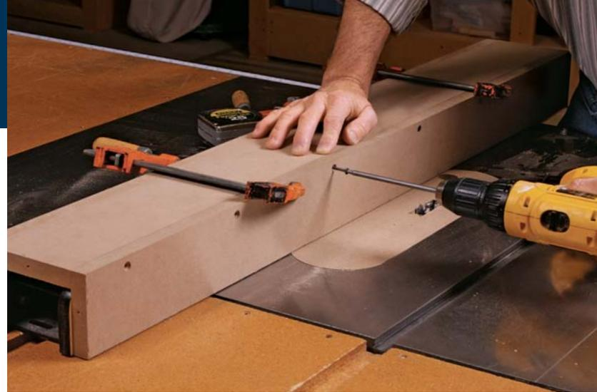
**How to get a snug fit.** Cut the sides 1 in. taller than the rip fence, and long enough to allow clearance for the lever at the end. Clamp the sides in place to measure for the top plate and attach it as shown. Drill pilot holes to prevent splitting. Keep the clamps on as you screw on the end caps.
