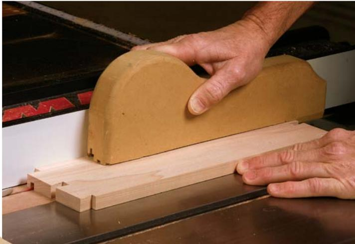
**Ride the fence.** Adams makes grooves with a single blade, making multiple cuts for wider grooves. A long push stick gives better downward pressure and control.
