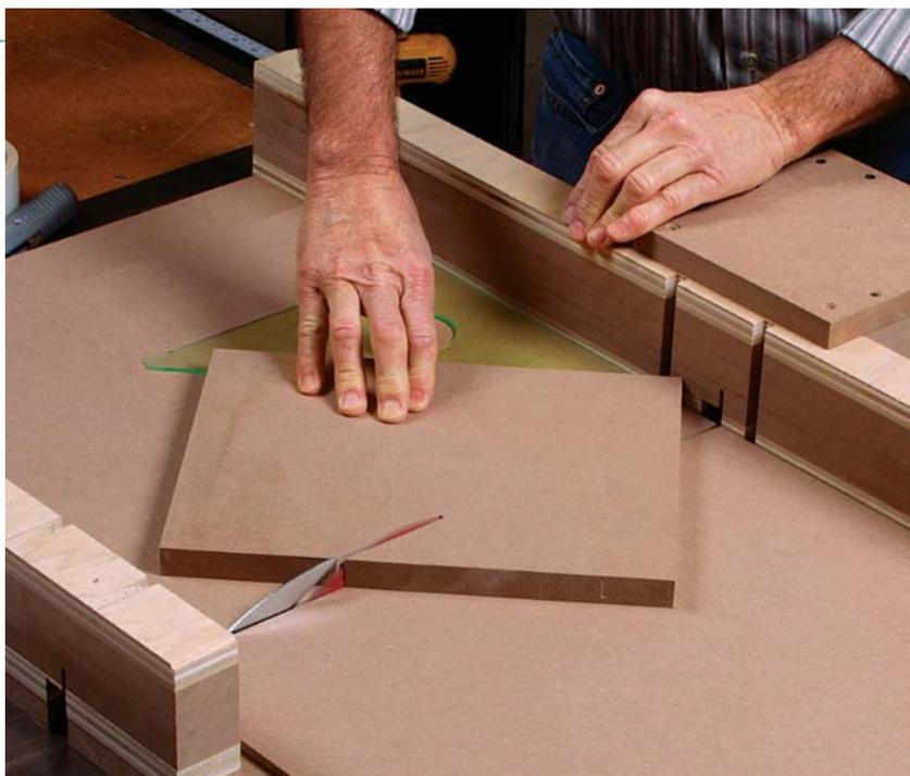
**Easy to make.** Use a 45° drafting triangle to position the MDF fence on the sled. Use carpet tape to hold it down, but keep the triangle in place as you cut, to be sure the workpiece doesn't shift.
