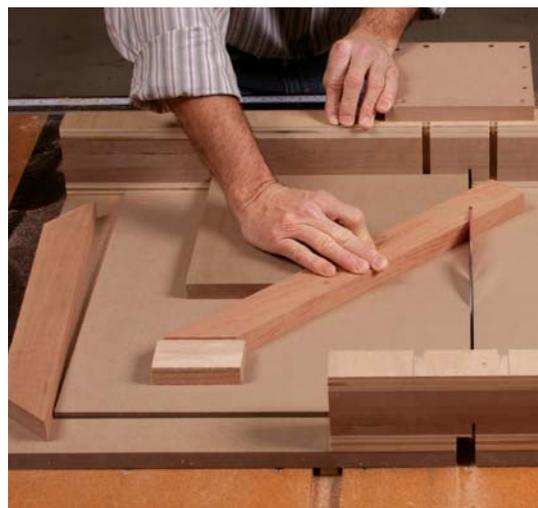
**Switch sides.** Flip the fence over to set it up on the other side. This time you'll need a stop to set the final length of each piece, but that's as simple as taping a block to the sled. The miters should come out perfect.
