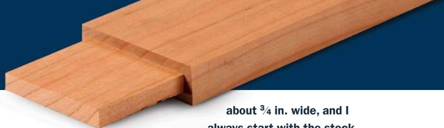
about  $\frac{3}{4}$  in. wide, and I always start with the stock against the rip fence for the first cut and then nibble away the rest. Do not lift the stock when you finish a cut; just keep a tight grip as you pull it back.
