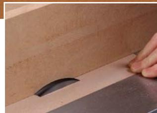
**Add the fence and bury the blades.** Use thick carpet tape to attach a tall MDF fence (above), then move the fence over the top of the dado set and bring the spinning blades up into it (left), only as high as needed.
