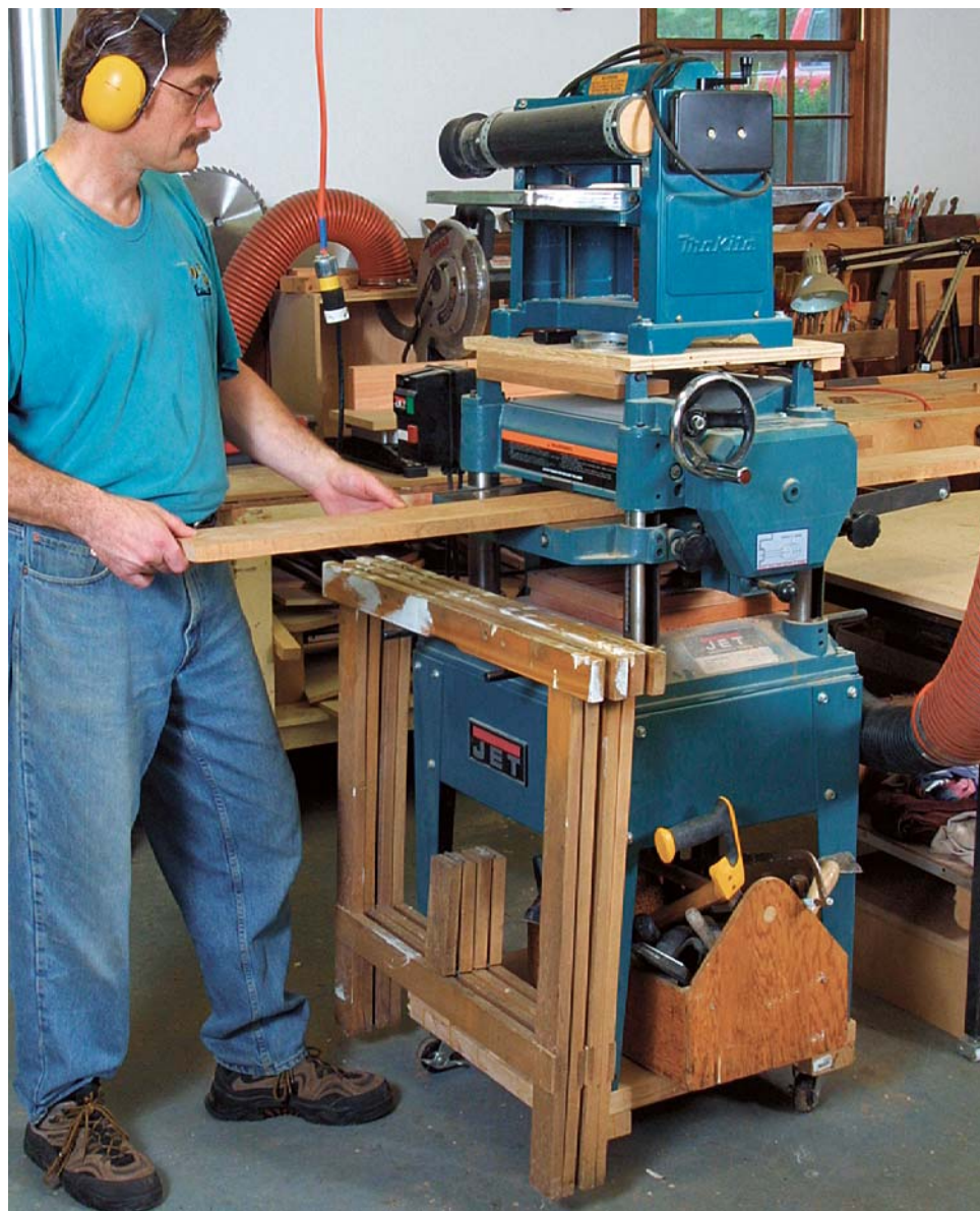
Machines to surface stock. The 15-in. planer can remove stock quickly. The benchtop planer riding piggyback excels at taking light passes without leaving knife marks. And a drum sander (not shown) speeds up what most consider the least enjoyable part of woodworking.
