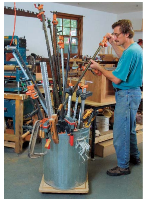
Clamps to go. Stored in a metal trash can, clamps can be wheeled to the assembly area, then rolled into an out-of-the way corner when not needed.
