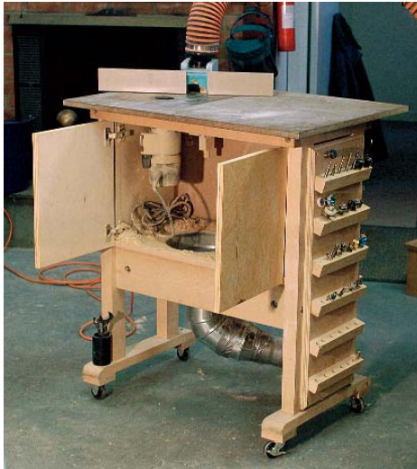
Traveling router cabinet. Dust collection is provided below, via a 10-in. to 5-in. reducer, and above, via a 2½-in.-dia. hose connected to the fence. The table is big enough to add another router if needed.
