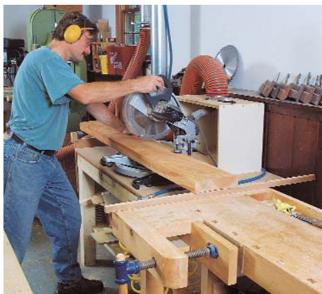
Sawdust is captured by a box, which is connected to the dust collector. A roller bolted to the left of the table provides stock support. The workbench (with the aid of a piece of scrap) provides support to the right of the chopsaw.
