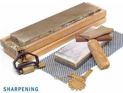
For the inevitable sharpening, Rodriguez prefers waterstones. But he also carries a coarse diamond stone for quick removal of dings and chips in tool edges. A honing guide speeds up the process.
