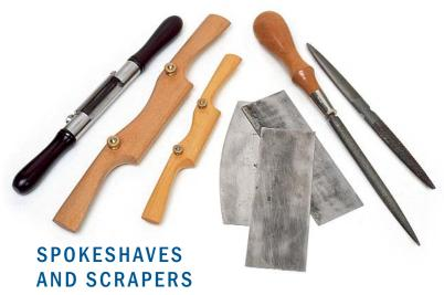
Rodriguez packs three spokeshaves; the smallest has a 1½-in.-wide blade. Flat card scrapers take up virtually no room but are versatile performers for smoothing surfaces and removing plane marks. The Grobet detail file and Italian rasp are used for cleanup and shaping.
