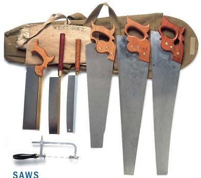
Used for joinery and cutting stock to size, handsaws are essential travel companions. They include (from left): a backsaw, two dovetail saws, two crosscutting saws and a ripsaw. A jeweler's saw (bottom) is useful for cutting veneer inlays and for removing waste from dovetails.
