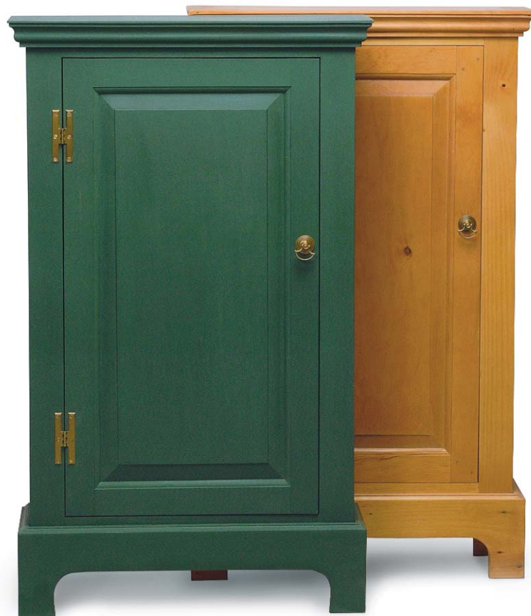
Options, options. At far left is the cabinet finished with Lexington Green milk paint, with a linseed-oil overcoat. The other version is finished with four washcoats of concentrated tea followed by a tinted shellac.
