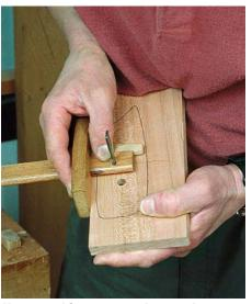
Use a marking gauge to lay out the sides. A %-in.-dia. hole defines the rounded end. The mortise extends from the edges of the hole.
