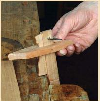
Fine adjustments are made with one hand. Light taps on the benchtop adjust the arm, and another quick tap tightens the wedge. It takes a little experimentation to get used to the interplay between the two parts.
