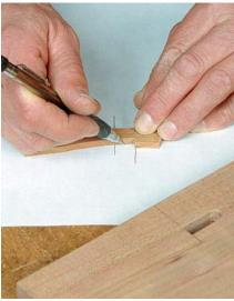
Then overlay the wedge to trace a cross section of the mortise needed. Use the narrowest portion of the wedge.
