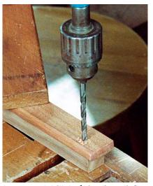
Lay out and drill the 1/4-in.-dia. relief hole. With the center relieved and only the front and back of the slot to worry about, the blade will be easier to fit.
