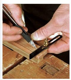
The slight angle is critical to the tool's cutting action. The thin slot is laid out 3° or 4° off square, but it will be square vertically through the arm.
