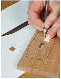
The resulting paper block now contains the exact lengths of each side of the angled mortise. Lay out each side and chop out the mortise.
