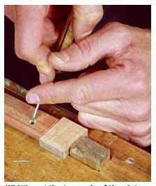
Whittle out the two ends of the slot, fitting them to the blade. Only  $\frac{1}{2}$  in. of the blade should protrude from the bottom of the arm.
