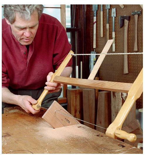
When the arm and wedge mortises are complete, cut out the arm and fence. The author shapes the roughsawn parts with hand tools, using a shallow gouge and a block plane.
