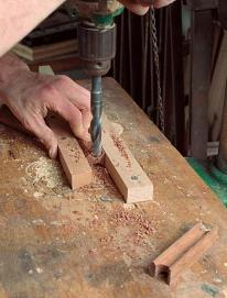
**Production sequence for a lot of matching pulls.** Coved sides, held down firmly with a push stick, can be cut in long lengths on the router table. After individual pulls have been cut to length, the author uses a drill bit (matched to the size of the cove, mounted in a drill press and fitted with a stop block) to cut the same coves on the ends of the pulls.
