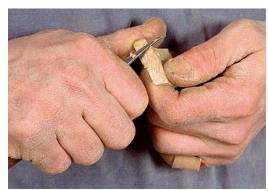
**Hand and machine work combine to do the job.** After cutting this pull to rough shape on the bandsaw, gouges, rasps and carving knives are all required to complete what is essentially a handcarved pull.
