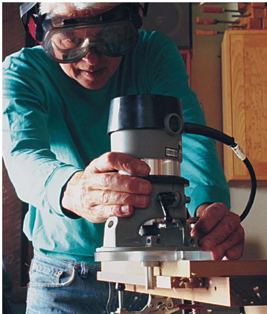
**Collars have the edge.** A collar and a perfectly straight, simple template can help a straight or spiral bit put a finished edge on long grain or end grain.
