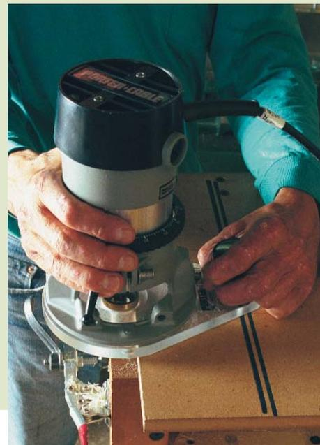
**An offset subbase is a good idea.** An offset subbase will help steady a router with a collar attached. You can correct for any lack of concentricity in the collar by keeping the collar against the template. Do this by drawing a line on the template and guiding the subbase handle along that line.
