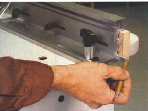
The Bench Dog has aluminum rods for shimming the outfeed fence . One face has been machined to square it up. Also, large knobs are used for all adjustments.
