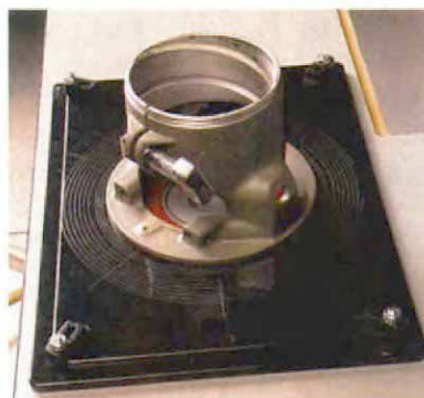
Rousseau's concentric rings help align a router prior to drilling mounting holes. Getting a router perfectly centered is possible, but you must have a good eye.
