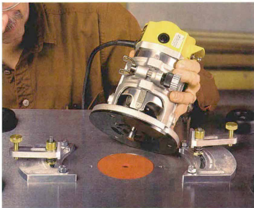
The Veritas router table comes with an alignment pin for centering the router in the baseplate hole. The unique clamping system doesn't require the user to drill any holes or to remove the router's subbase to mount the tool.
