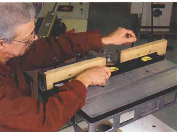
A fence should be square to the table and easy to adjust. A split fence, which is found on many benchtop models, such as the Woodstock Rebel, must be realigned each time it is moved, a time-consuming process.
