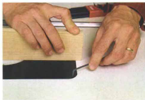
Levelers are built into the Eagle America baseplate. Six Allen screws are easily adjusted from above.
