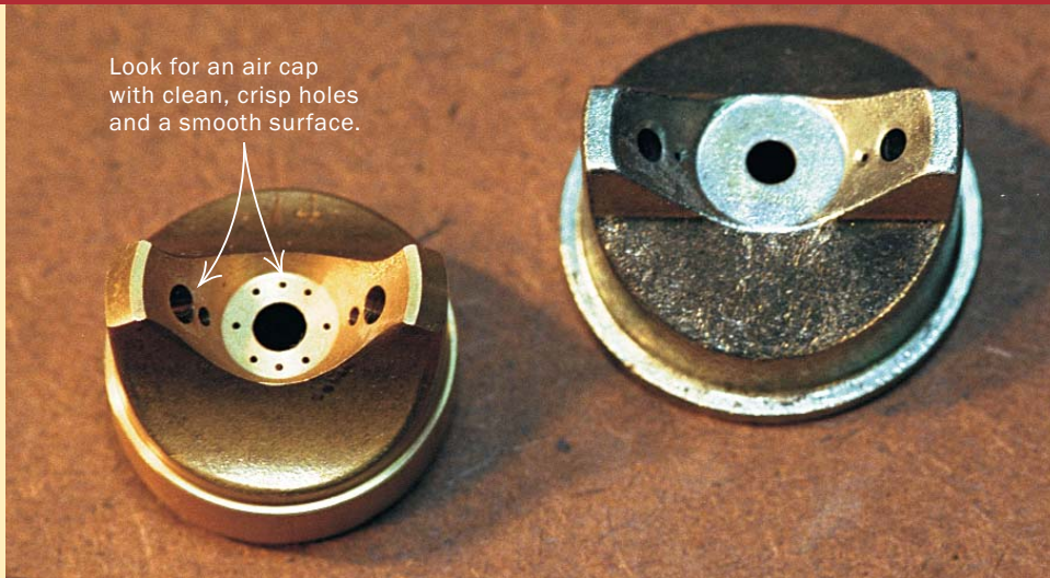
Which air cap delivers a better finish? A well-machined air cap, such as the Lemmer (left), had a more efficient spray pattern with less overspray than the Campbell Hausfeld cap (right).
