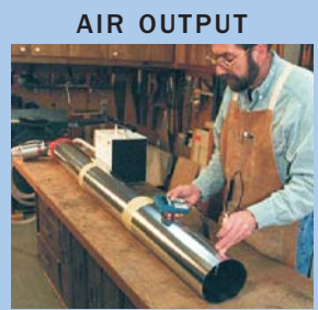
Measurements of actual air output, made with an anemometer, did not agree with those of most of the manufacturers.
