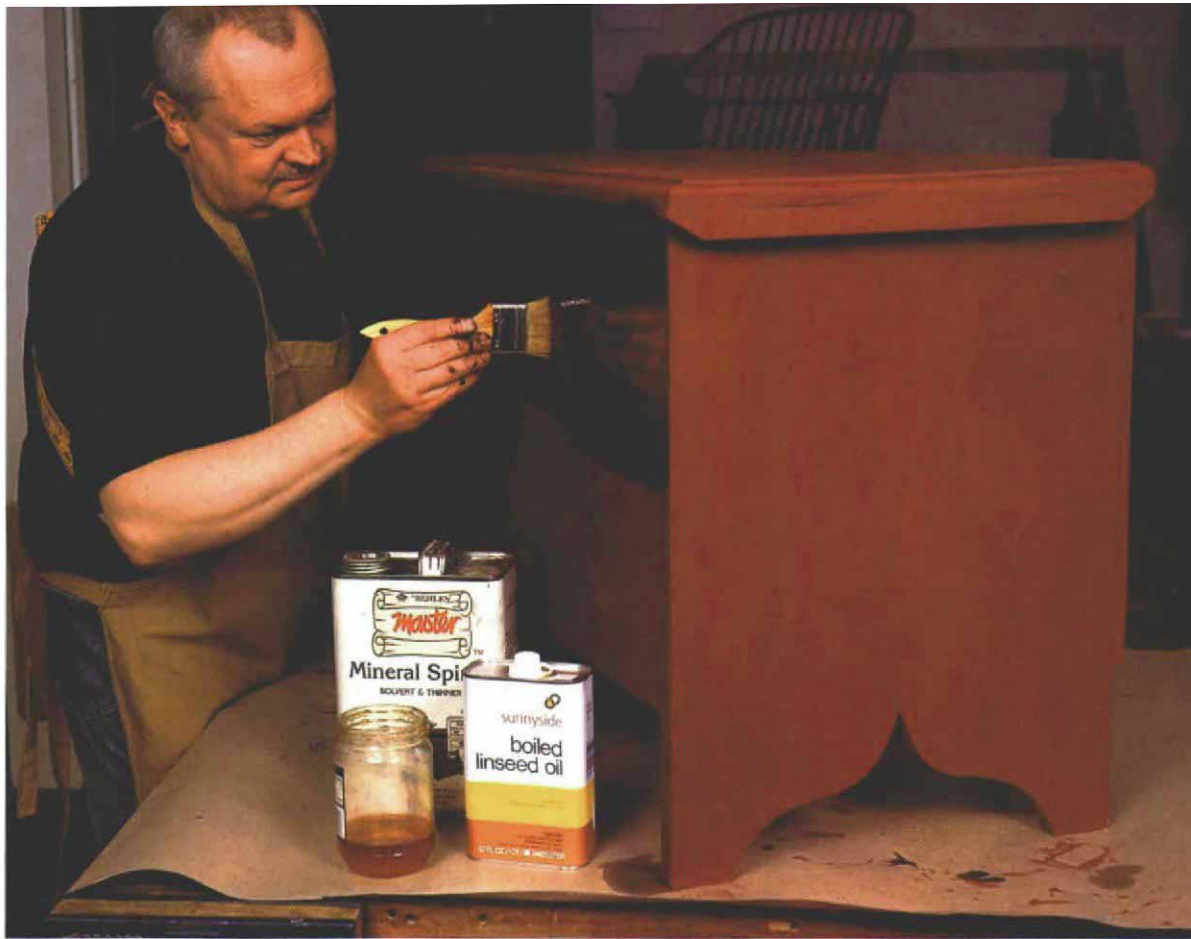
Thinned linseed oil over flat paint. A mixture of five parts boiled linseed oil and one part paint thinner is brushed on as a final coat. Excess is wiped away with a lint-free rag.
