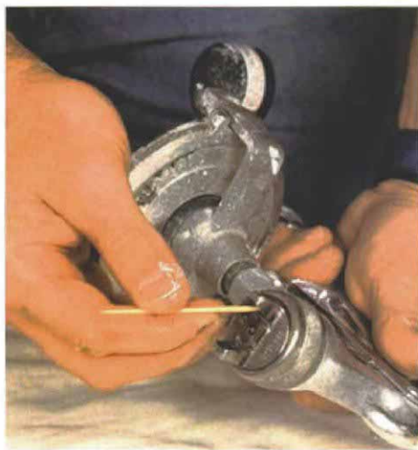
Clear the air passages. Wood toothpicks won't damage the precisely machined air-cap orifices, which can get clogged with finish.
