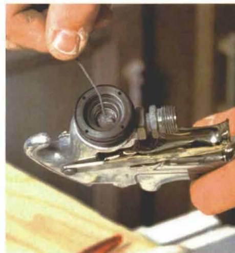
Remove the air cap and fluid nozzle. The inside of the gun is best cleaned with a skinny brush soaked in lacquer thinner.
