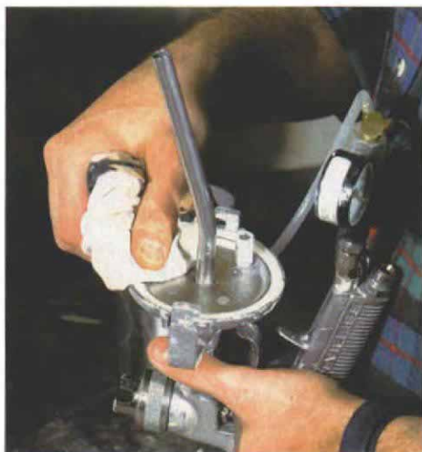
Clean the gasket. The gasket needs to be free of debris; otherwise, the gun will not seal properly and will leak when tipped.
