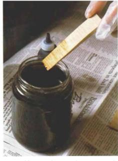
step. I dilute it eight times the recommended concentration, or until it's the color of strong tea (see the photo above). After sanding the wood through 150-grit paper, lay on this dye as a grain-raising step. Wipe or spray it quickly all over the wood as evenly as you can, then let it dry. Sand the raised grain with 180-grit paper. Sanding will remove almost all of the dye color
