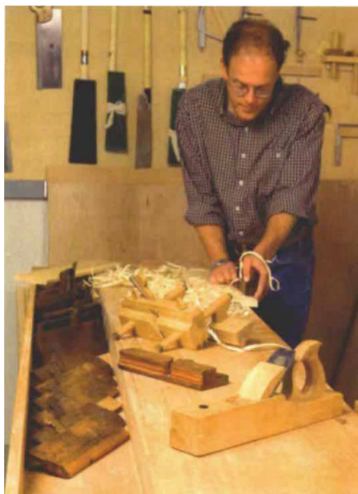
For planes and benches, beech is best. Beech is long wearing, dense, shock resistant and abundant, qualities that have made it the enduring wood of choice for the majority of wooden planes and workbenches.
