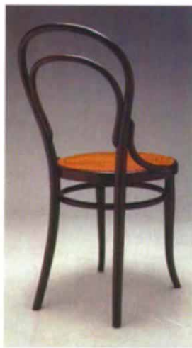
Beech bends beautifully. A Thonet chair made in the 1860s illustrates the pliability and durability of steam-bent beech. By utilizing only small-diameter parts, the chair also minimizes the effects of beech's excessive seasonal movement.
