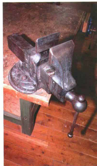
Smooth operator. This antique Prentise vise (right) has smooth faces that won't mar wood.
