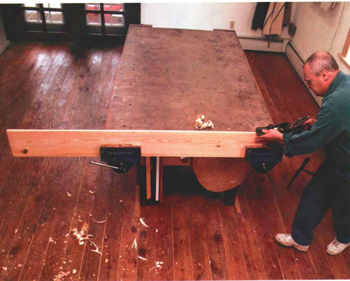
Smooth operator. This antique Prentise vise (right) has smooth faces that won't mar wood.
