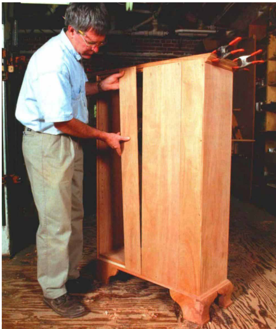
Shiplapping allows solid boards to move. A single screw placed near one edge of each board (at top and bottom) will enable each rabbeted board to hold down the board next to it, while allowing each board to move with seasonal changes.
