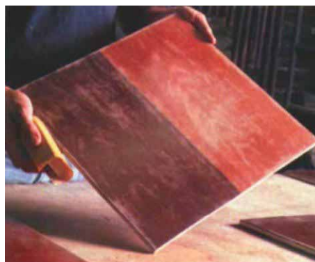
Too-thin finishes are tricky to sand. Some finishes, such as J.E. Moser's Cool-Lac, a water-based shellac, go on so thin that it's difficult not to sand through to previous coats.
