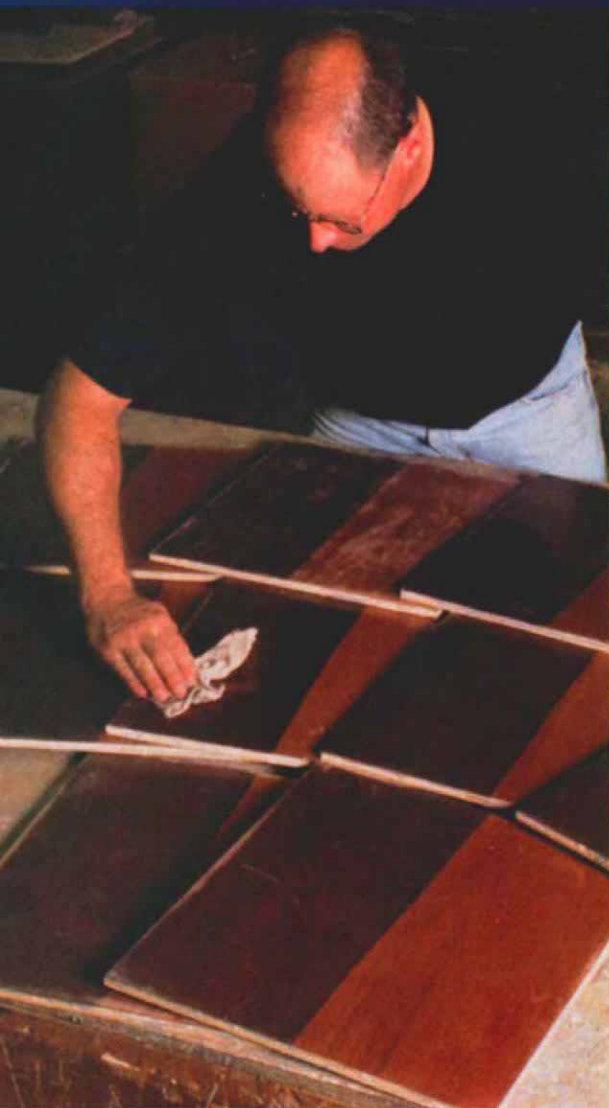
Finishes were tested on mahogany plywood. The author applied an oil-based stain to half of each panel, then three coats of finish.
