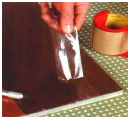
Testing adhesion over an oil-based stain. A sharp knife was used to slice into the finish, then packing tape was placed over the cut. After five minutes, the tape was pulled off.
