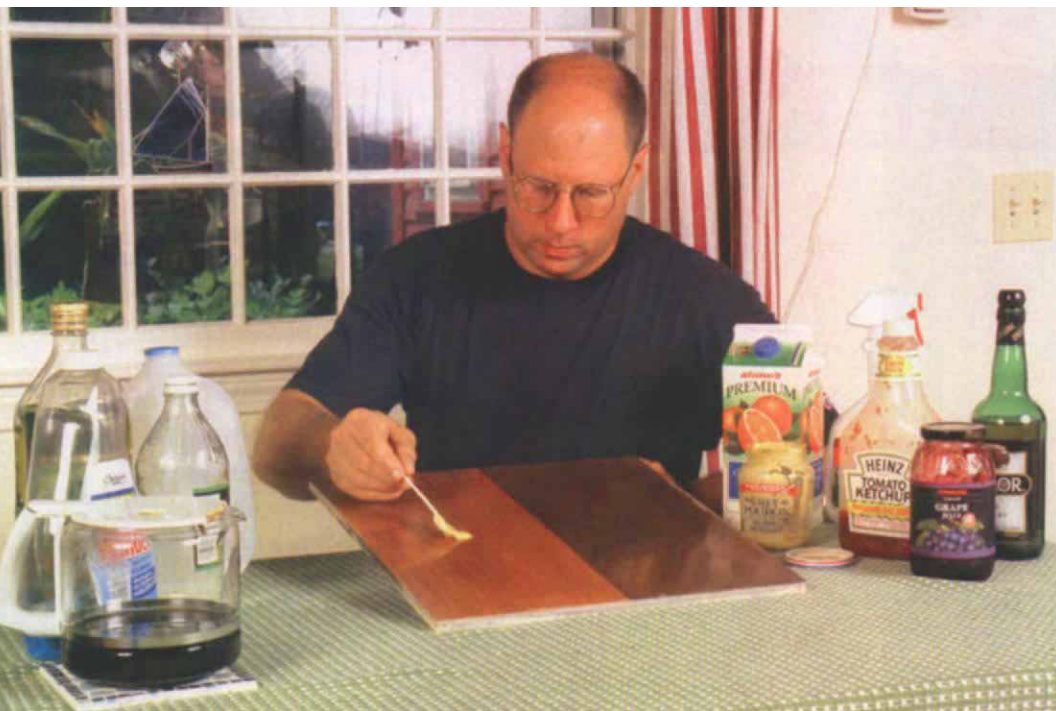
Food-stain test. Finishes were subjected to a variety of common foods and cleaners. Most finishes held up very well. Cleaning products, however, were hardest on the finishes.
