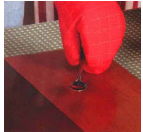
Hot-spoon test. Several finishes were marred when a hot spoon was allowed to cool on the panel.
