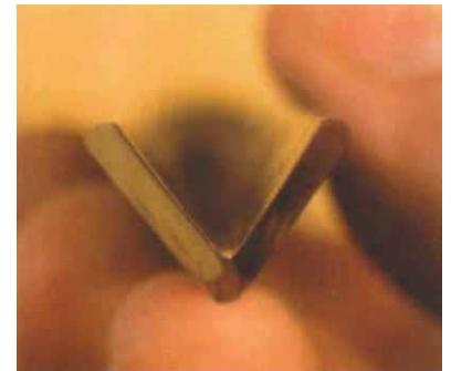
Looks sharp. A properly sharpened V-parting tool as seen from the front. Note the slightly rounded bottom edge.
