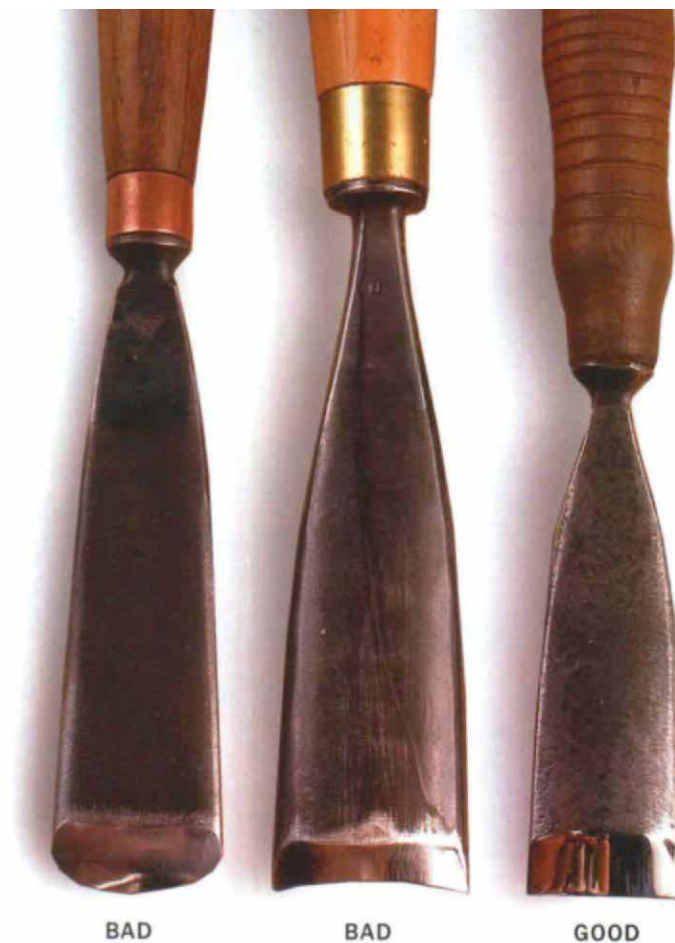
The edges of most carving tools should be square. Gouges with convex (left) and concave (center) edges will give you fits when carving. A square edge (right) provides the best control.
