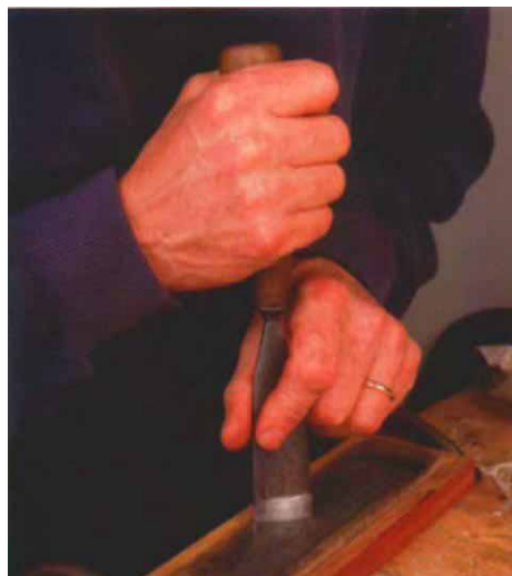
Grind a crooked edge square. Hold the tool vertically, and rub it back and forth across a stone, maintaining a 90° angle.
