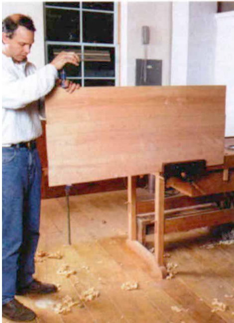
Garrett Hack glues up tabletops using his bench vise. With one board clamped in the vise, he applies glue and stacks the remaining boards in place. Next he applies bar clamps, beginning at the outboard side of the workbench. At the halfway point, he repositions the panel in the vise, allowing the clamps to rest on the floor for support. The remaining clamps are applied with only about 1 in. of the panel gripped by the vise.
