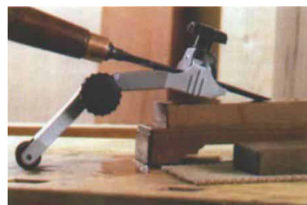
The General is the only guide that rests on and off the stone. The tool is hinged so it can be adjusted for stones of different heights.
