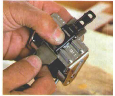
A built-in angle guide makes it easy to position a tool to this guide.
