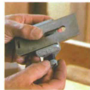
Each half of the guide has a pair of jaws: one for wide tools and another for narrow ones.
