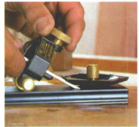
A large, easy-to-tighten hold-down knob and a wide roller make a secure, stable honing guide. An angle-setting gauge with five presets can be purchased separately.
