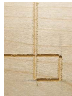
A router cuts the grooves. A \frac{1}{16} -in. straight bit and an edge guide on the router help make grooves of uniform depth. They still must be cleaned up.
