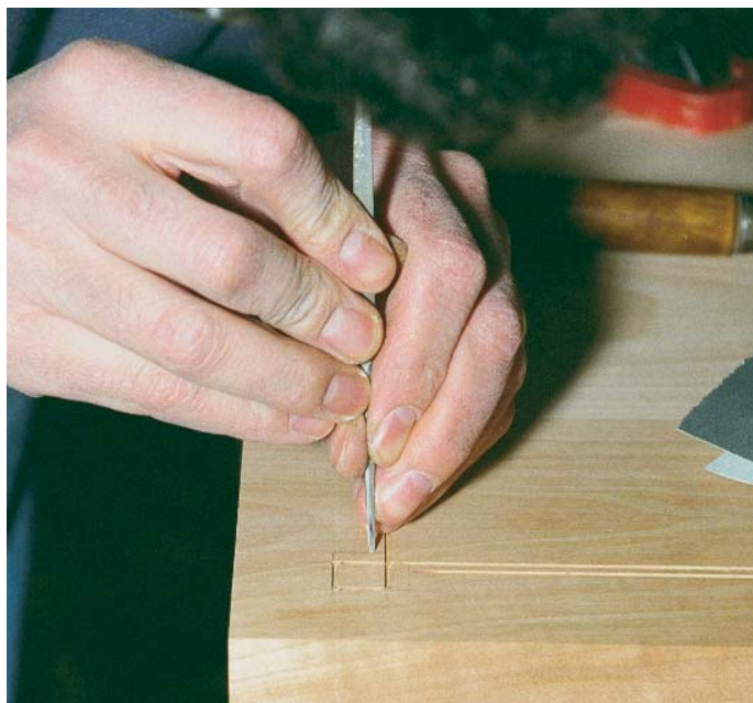
Clean grooves carefully before trying epoxy. The end of a small file ground to form a narrow chisel squares up corners. Fuzzy edges and the bottoms of the grooves should be cleaned up with 320-grit sandpaper.
