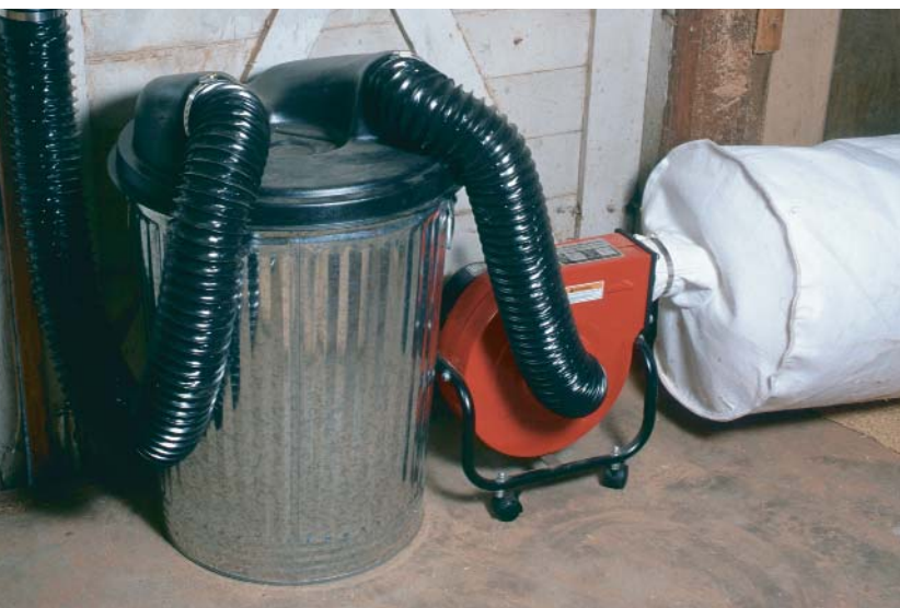
A built-in cyclone does an excellent job separating chips and dust before they reach the blower. This Delta 50-903 collector has a 5-hp motor.
