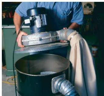
The lid can be heavy with this kind of two-stage collector. One option would be to install a block and tackle nearby with a wall cleat to tie off the rope.
