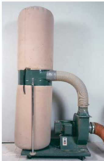
Single-stage collectors, such as this 2-hp unit, connect easily to small central-collection systems. One drawback is that the debris enters through the unit's blower where cutoffs or stray bits of metal can cause problems.
