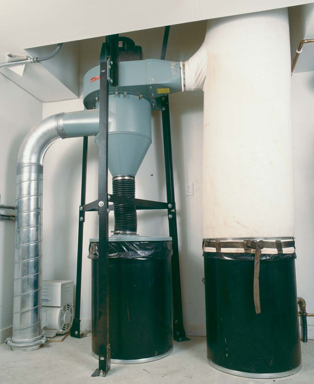
A built-in cyclone does an excellent job separating chips and dust before they reach the blower. This Delta 50-903 collector has a 5-hp motor.
