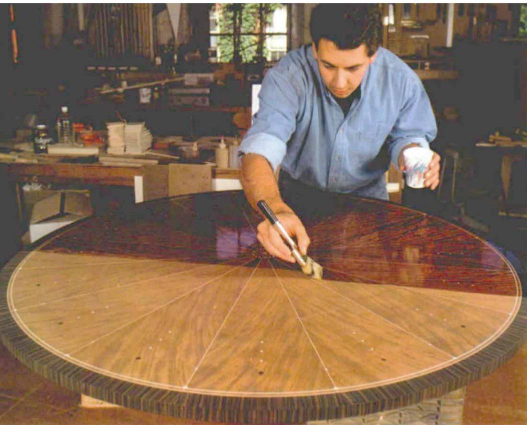
**Brush on the varnish in long, smooth strokes (left).** On a surface with a single or a predominant grain direction (unlike this sunburst veneer pattern), start by applying the finish across the grain. The first coat of varnish should be a 50/50 solution of varnish and solvent.
