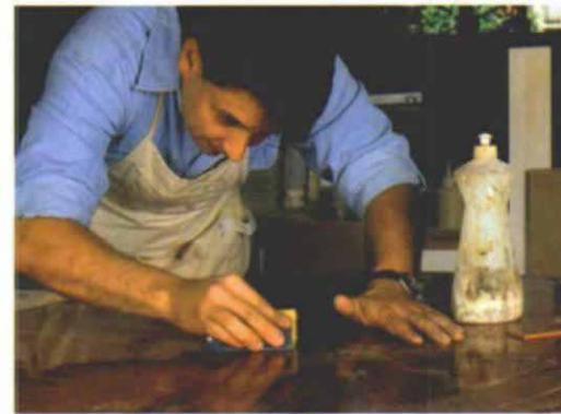
**Rub out nubs or bumps with 1,200-grit paper wrapped around a wooden block (above).** Water, naphtha or mineral spirits may be used to lubricate the surface.
