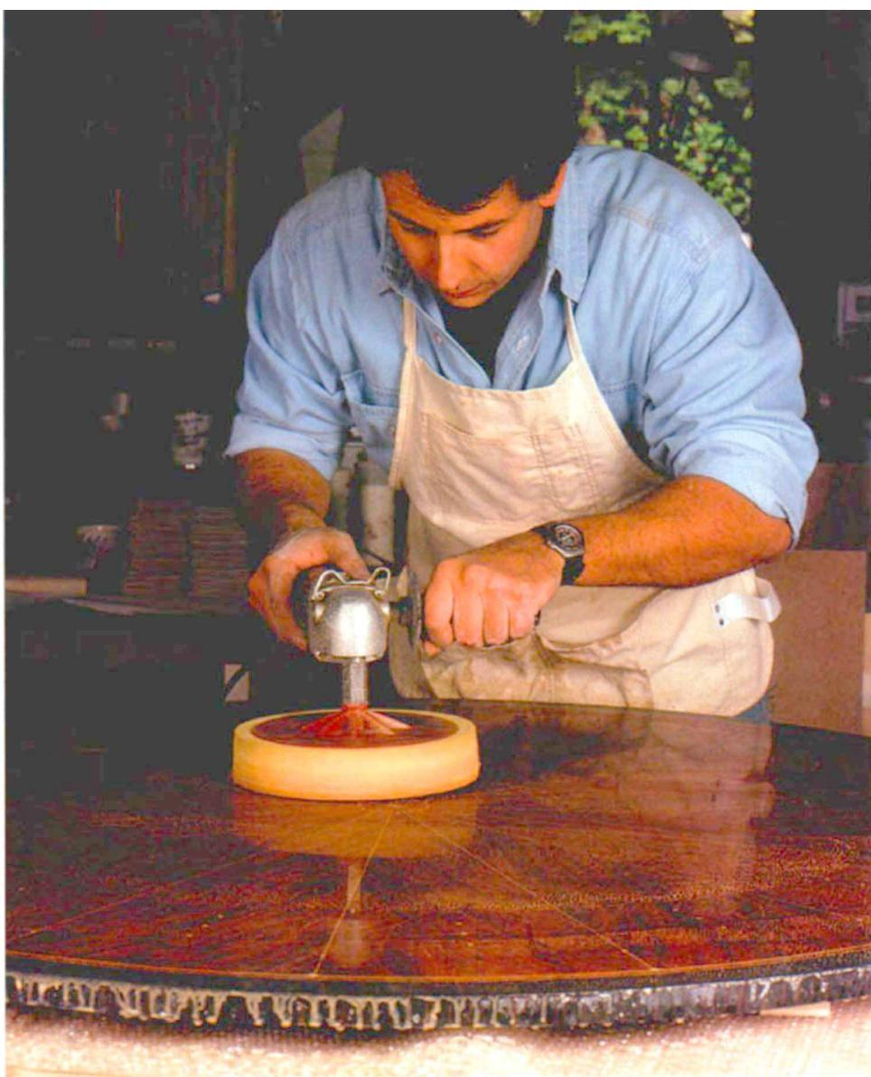
*Polish the finish with a power buffer and automotive glaze. Once you've sanded out all the nubs and bumps and gotten the surface flat, 10 minutes of power buffing will take the finish to a high-gloss shine.*
