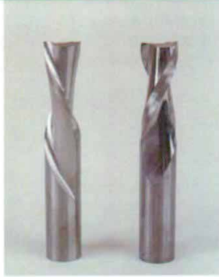
Spiral flute cutters slice wood fibers. The down-shear bit (left) leaves a crisp edge at the top surface. The up-shear bit efficiently ejects chips.
