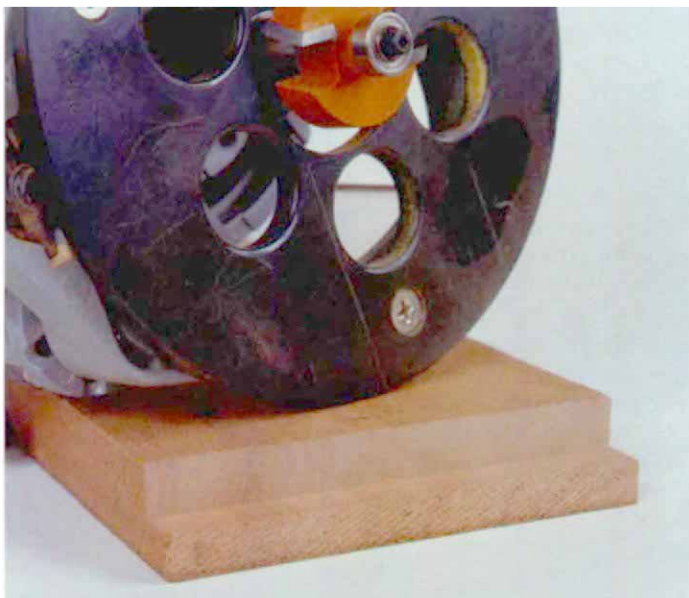
Shear angle reduces tearout on end grain. The angled cutter on this rabbeting bit cuts cleanly in redwood.
