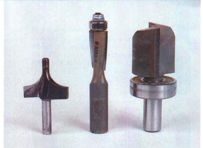
Pilots guide bits for uniform cut. The solid pilot on the end of the bit at left spins against the stock and leaves burn marks. The ball-bearing pilots on the center and right bits eliminate burning.
