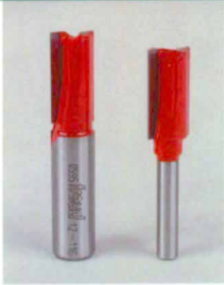
Both bits make a cut 1/2 in. wide, but the 1/2-in. shank (left) reduces chatter and allows a more aggressive cut than the 1/4-in. shank bit.
