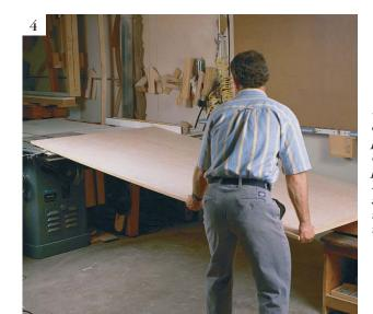
1. Platform is at a comfortable height for unloading. The author slides plywood from his truck to the platform and tilts the panels up to the stack. He doesn't have to lift the full sheet.
