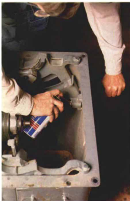
White lithium spray grease is used to lubricate the hard-to-reach pivots.
