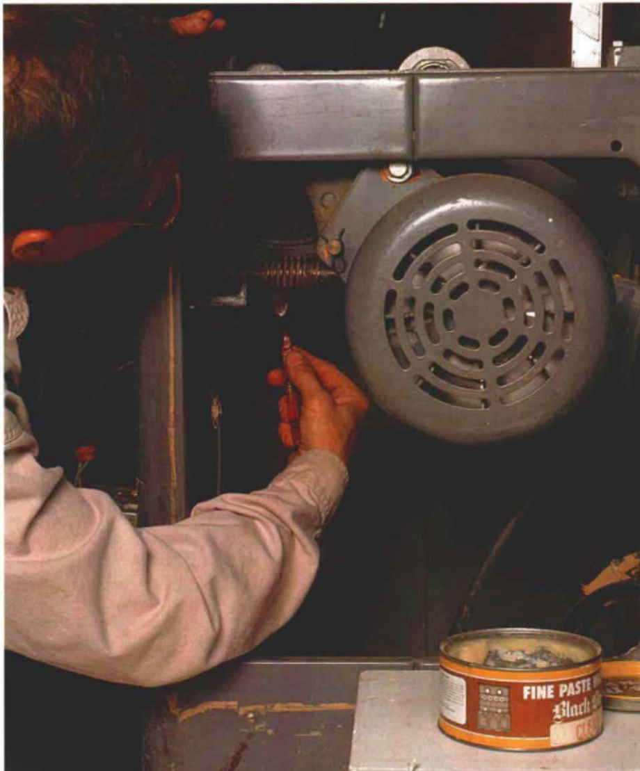
Paste wax applied with a toothbrush lubricates gears and doesn't attract sawdust.
