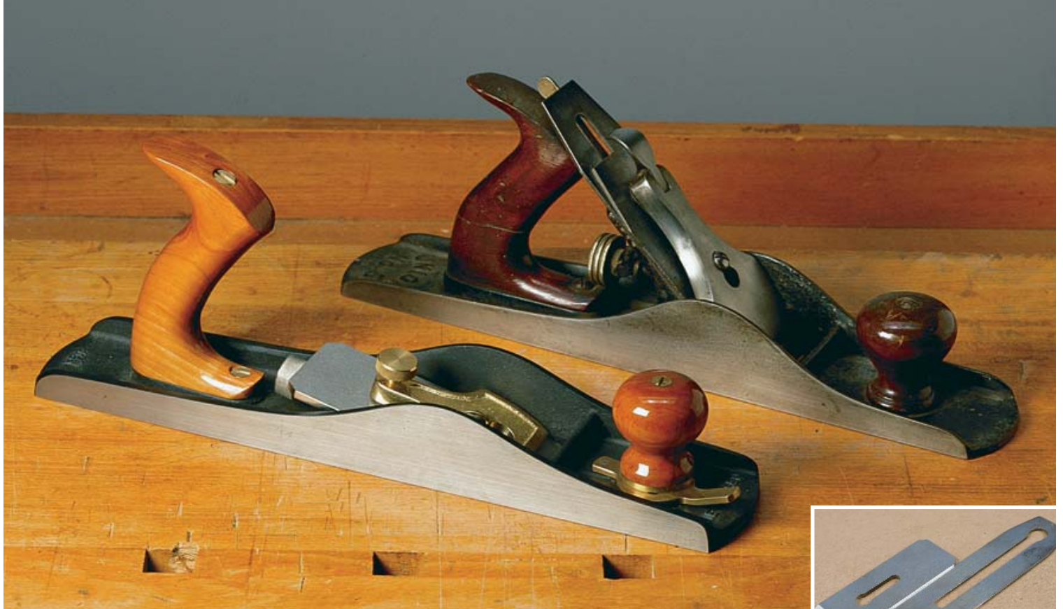
These planes are cousins, not twins. A Union No. 5 plane (rear) and a low-angle jack plane from Lie-Nielsen show similarities but big differences, too. The Lie-Nielsen delivers high performance at a high price. The Lie-Nielsen blade (see inset photo) is thicker than the Union's.
