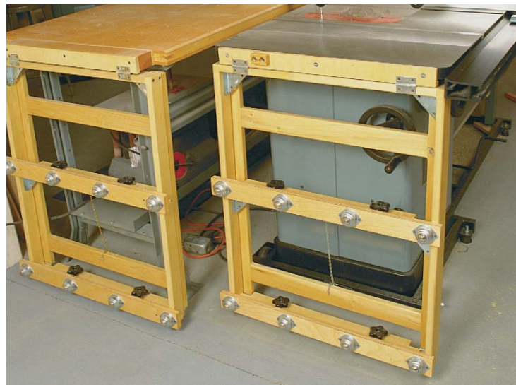
The extension table drops into its stored position in seconds and takes up no floor space. Adjustable roller assemblies can be raised so that the table also works with a sliding crosscut box.
