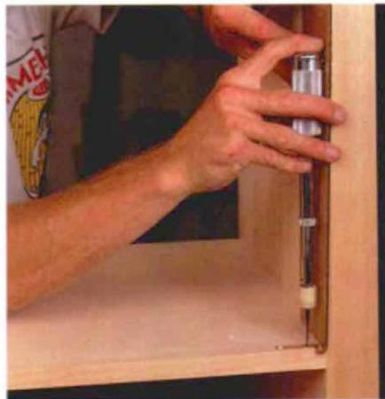
**Drill suited to a tight spot.** A Yankee drill lets the author drill screw holes against the carcass's side. This would be impossible with a power drill or a corner brace. A piece of cardboard prevents the side of the carcass from being marred by the drill.
