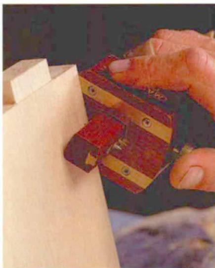
*Marking-gauge line establishes front edge of mortise. Scratch a marking-gauge line from pencil mark to pencil mark. The marking gauge should be set for the distance from the center of the pivot pin to the outside edge of the hinge leaf's long leg. Try not to let the gauge wander along any sloping grain.*
