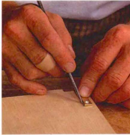
**Mark back side with a knife.** Tilt the hinge leaf into the mortise, and hold it tightly against the front wall of the mortise to mark the back edge. Then pare carefully to this knife line, checking frequently to see if the hinge leaf will fit. Once it fits, that mortise is done. The procedure is the same for all four mortises.
