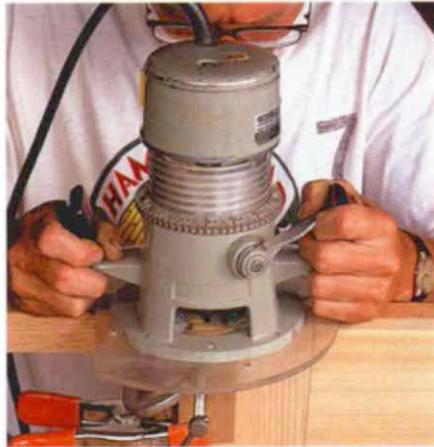
**Cutting mortises in the door.** A board clamped to door gives router a steady platform. Otherwise, routing the mortise in the bottom edge of the cabinet door would be a tippy proposition. Be sure to use clamp pads (here held in place with spring clamps) to avoid damage to the door.
