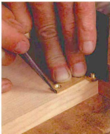
*Use a knife to mark edge and end of mortise. Position the hinge leaf on the marking-gauge line, mark the end of the hinge leaf and the inside edge of the "L" with a knife, and then erase the pencil lines.*
