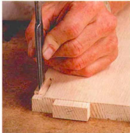
**Clean up roughness left by router along back edge.** With a chisel, the author removes most of the waste remaining in the mortise. But take care to stay well away from the pencil line—the back edge still needs to be marked with a knife.
