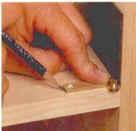
*To lay out the hinge mortise, start with a pencil. With a laminate shim between the carcass wall and the hinge, the author marks the end of the hinge leaf and the edge of the short leg of the "L." These reference lines set limits for a marking gauge, which is used next.*
