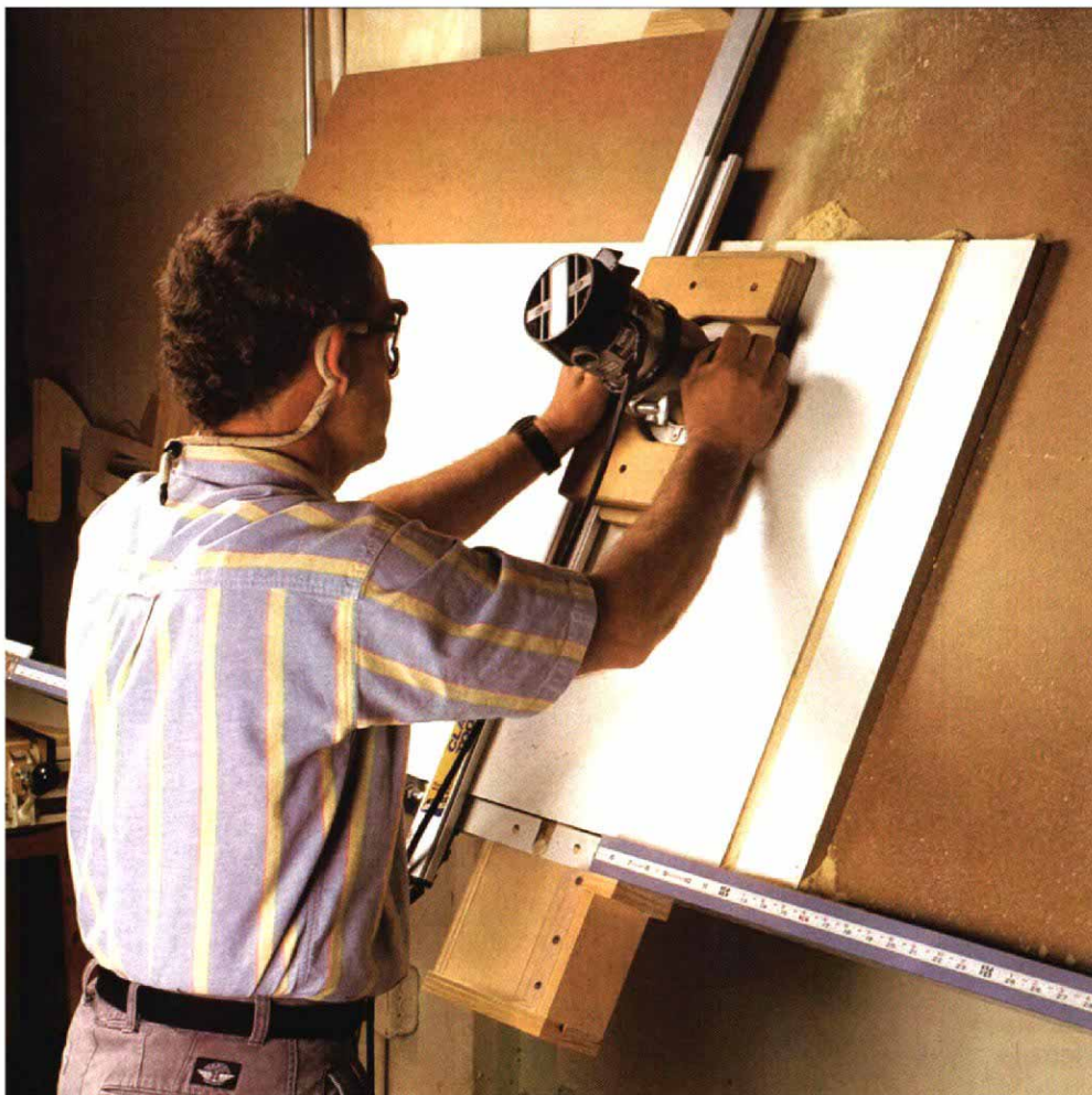
Wall-mounted panel router is ideal for making quick dados. Knowing his panel router had to save space, Skip Lauderbaugh mounted it to a wall at a comfortable height and angle. To build the jig, he used a router he owned and commercial hardware costing less than $100.
