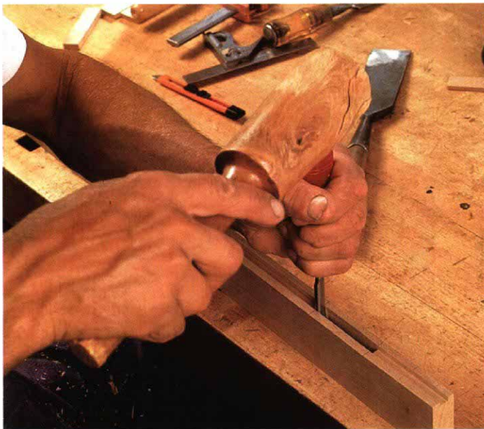
Fig. 2: Mortised-and-tenoned breadboard technique
