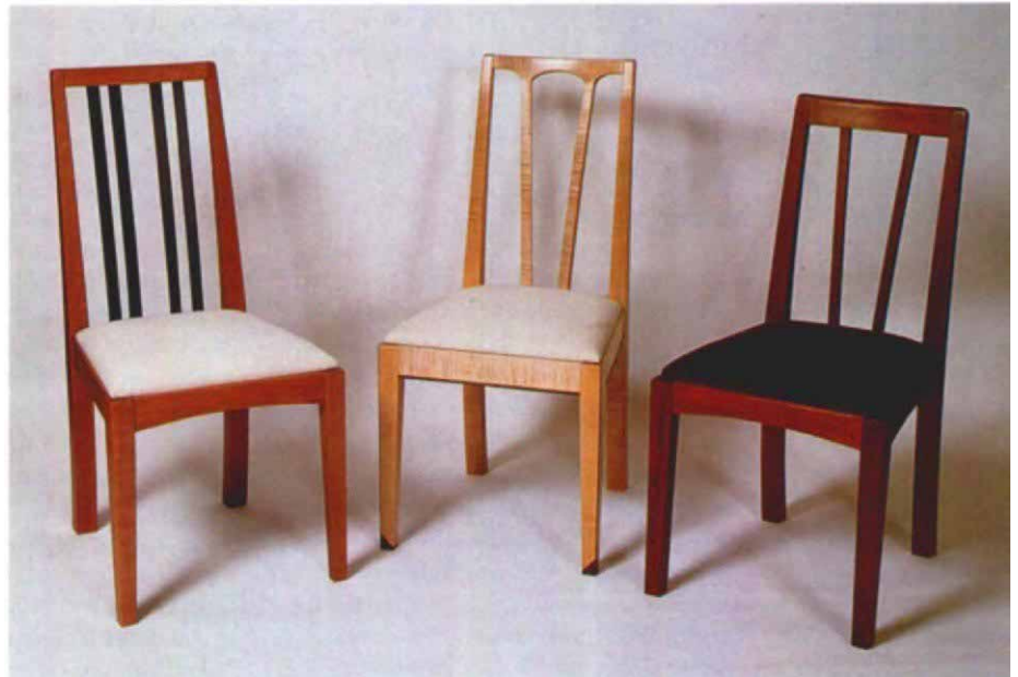
These chairs are from the same design series developed by Moore. Although each is different, they all share the same construction methods based on a series of shop-built patterns and jigs. The chair on the left is of Honduras mahogany, the chair in the middle is curly maple with rosewood inlay and the chair on the right is cherry with ebonized back slats.
