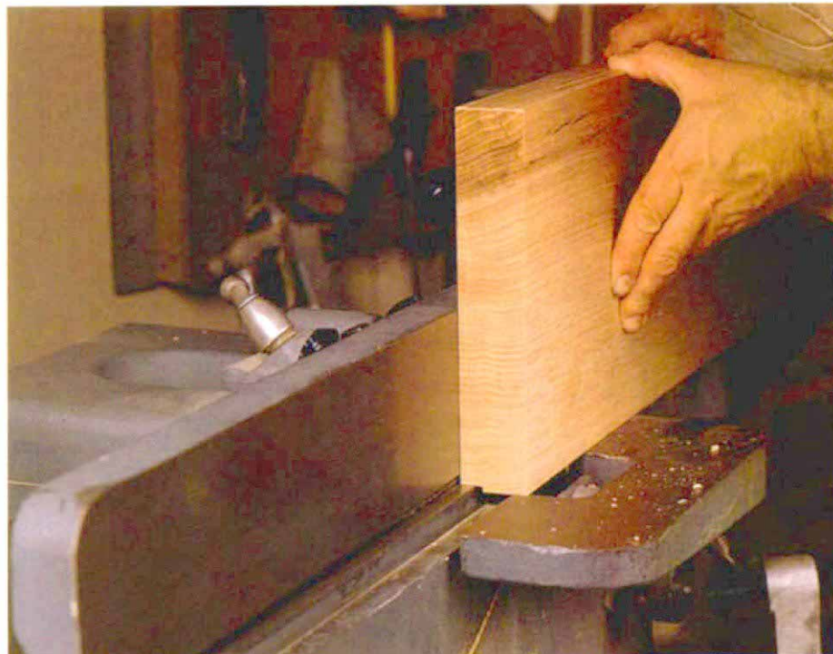
The rabbeting arm supports the board, and the notch in the outfeed table lets the unrabbeted portion of the board go by. Here the author is on his third pass; when rabbeting, the infeed table is lowered an additional \frac{1}{16} in. for each successive pass.
