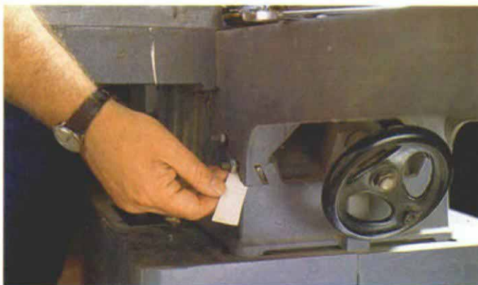
If adjusting the gibs fails to correct a table sag or tilt, brass or paper shims can be inserted as shown to lift the table.
