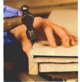
Carving is secured in the frame with finishing nails squeezed into place with a pair of pliers (above, left). The jaw on the outside of the frame is padded with tape to prevent marring. To reinforce and protect the carving, a plywood backing is nailed to the frame, as shown above, right.
