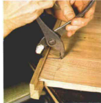
Carving is secured in the frame with finishing nails squeezed into place with a pair of pliers (above, left). The jaw on the outside of the frame is padded with tape to prevent marring. To reinforce and protect the carving, a plywood backing is nailed to the frame, as shown above, right.
