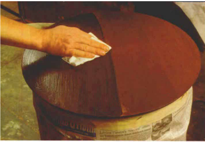
Glazing is done by thoroughly sanding the first coat of varnish and then wiping with an oil-based stain (above, left). Remove any heavy build-up before spraying additional coats of varnish. The subtle tone change obtainable is evident in the photo above, right.
