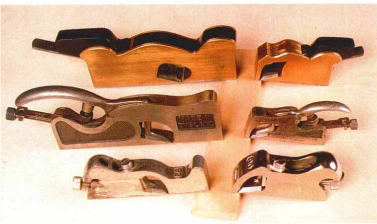
The chronology of shoulder and bullnose planes. Top to bottom: (19th- to mid-20th-century British), bronze and ebony Norrises; (20th-century British), Record #042, with depth adjustment, and Preston bullnose; and (20th-century American), Stanley #92, with adjustable blade and mouth, and Stanley #90 bullnose.
