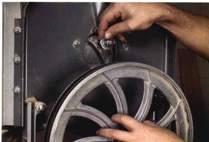
Slipping a regular \frac{5}{8} -in. hardware-store washer on the axle of the Delta bandsaw's top wheel shifts its position sideways to put it in plane with the lower wheel.
