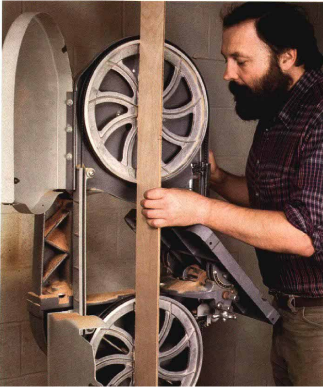
With the table tilted out of the way, the author uses a strip of plywood with a straightedge jointed on it to check the wheels of a Delta 15-in. bandsaw for plane and parallel alignment.
