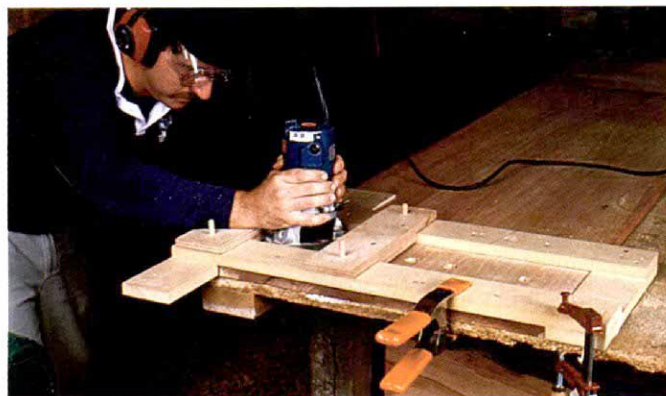
By changing the position of the two movable rails that guide the router, the author works his way across the bottom of the carcass side, chopping mortises for pin tenons that will join the sides to the bottom of his wardrobe cabinet.
