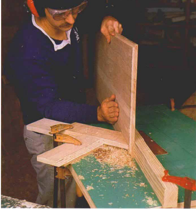
The author makes raised panels for the wardrobe doors on the router table. In the first step, shown above, he reduces the thickness of each panel's edge by running the panel vertically by a straight bit. A fingerboard clamped to a spacer provides the pressure needed to stabilize the panel as it's fed. This fingerboard also prevents the climb-cutting bit from self-feeding the panel.
