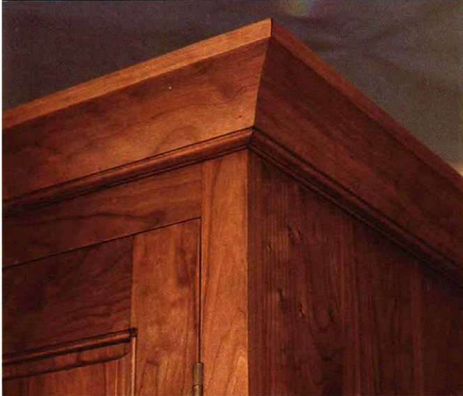
The beaded inner edges of the door frame and inlaid corners, as well as the cove-and-bead crown molding, provide the author's wardrobe with a distinguished degree of visual interest.
