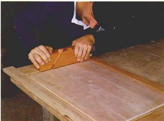
Hagood uses a homemade beading plane to detail the inner edges of the doorframe. The mahogany plane has two nonsymmetrical bead-profile blades, one for cutting in each direction. A piece of quarter-round molding on the underside of the plane guides it along the frame's inner edge for a straight cut.
