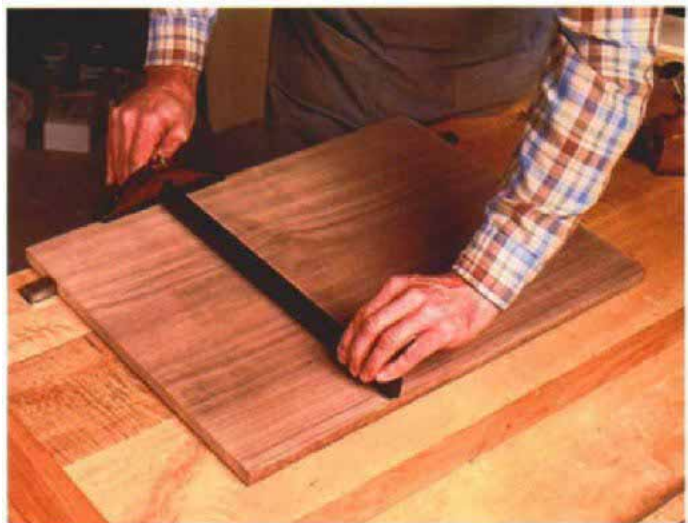
Although it's an uncommon marking tool, the panel gauge is handy for marking a panel or a wide board to be handsawn to consistent width. Two hands hold the long-beamed gauge for stability and to get a clean scribe line.
