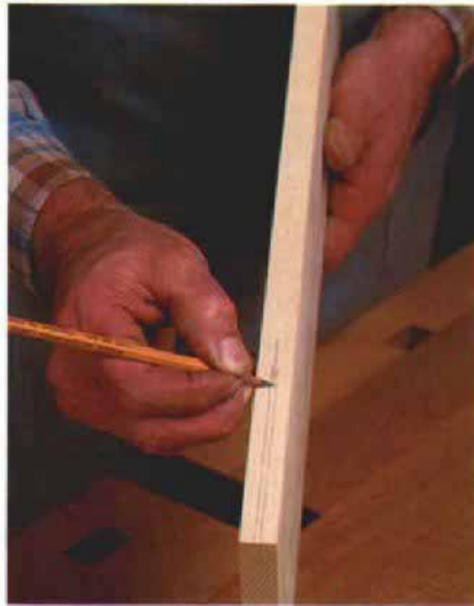
Using a tightly held pencil as a marking gauge, Klausz marks the board's center from both sides to find its center.
