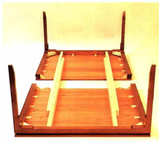
Extension tables allow many design options. Three-beam slides, as shown in the drawing above, can be fitted with a fifth leg to prevent sag. The author's long two-beam slides, visible in the photo below, have been tenoned into the table's aprons, thereby transferring load from the screws in the tabletop to the aprons and legs. Leaves can be aligned with dowels (see photo) or stub tenons (see drawing). Author de Rham's table and chairs are shown below, right.
