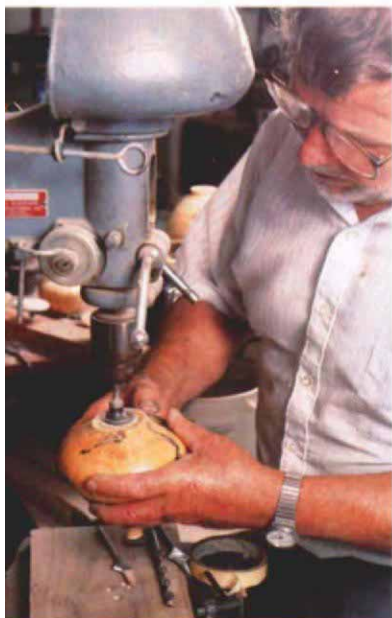
Sand bottom of the pot by rotating it freeband against a foam-backed sanding disc mounted on a mandrel cbucked in a drill press.
