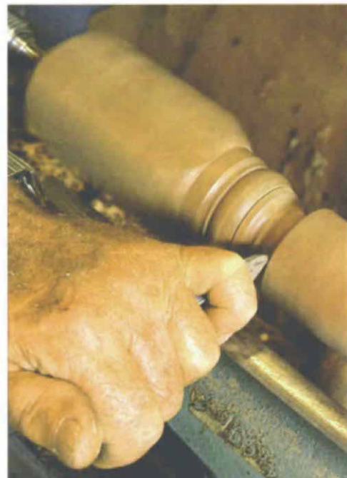
To cut the cove, right, roll the gouge down from each high point to hollow the section between the shoulders. Always cut downhill, toward the middle of the bellow.
