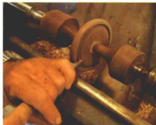
A walnut disc pressure-fit between two bottle-shaped plugs can be shaped to form bracelet. Free bracelet by working in hook-shaped tool, shown above, left, from both sides of disc.
