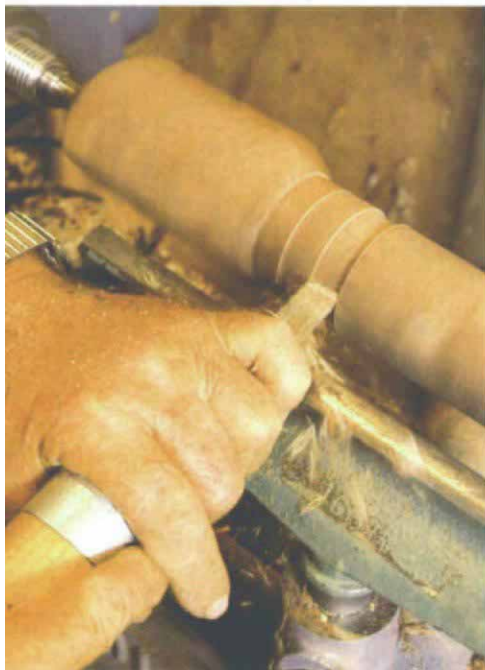
When shaping a spindle leg for a stool, use a parting tool to set the depths of the coves, left. After setting the depths, roll the gouge down each side of the flat band to create a bead, center.
