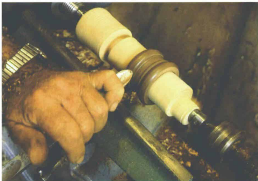
For a napkin ring, fit a block on a mandrel, left. Cut beads by rolling a gouge over the shoulders formed with a parting tool, right.
