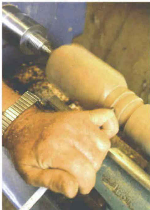
When shaping a spindle leg for a stool, use a parting tool to set the depths of the coves, left. After setting the depths, roll the gouge down each side of the flat band to create a bead, center.
