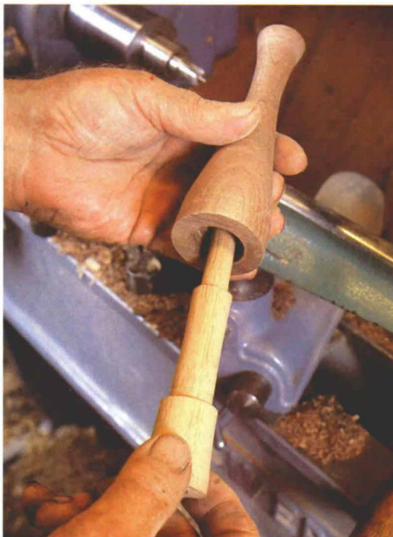
Turn plug to match three-stepped hole bored with modified twist drill, top. Hole could also be bored with three separate drills. Then, fit salt shaker blank on plug and mount it on lathe.
