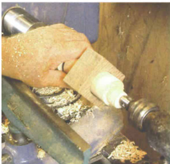
For a napkin ring, fit a block on a mandrel, left. Cut beads by rolling a gouge over the shoulders formed with a parting tool, right.
